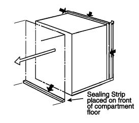
**NOTE:** Be careful not to damage the sealing strip applied to the floor of the enclosure when the refrigerator is put in place.
